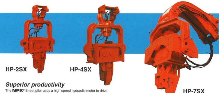
The **NPK®** Sheet piler uses a high speed hydraulic motor to drive two counter rotating eccentric masses developing powerful vibration forces. Vibration and shock loading to the boom and arm of the excavator is avoided by having the unit mounted in durable rubber cushions and the design of the sheet piler causes the impulse forces to be directed downwards, giving optimum driving of the pile and least vibration effects to the excavator.
